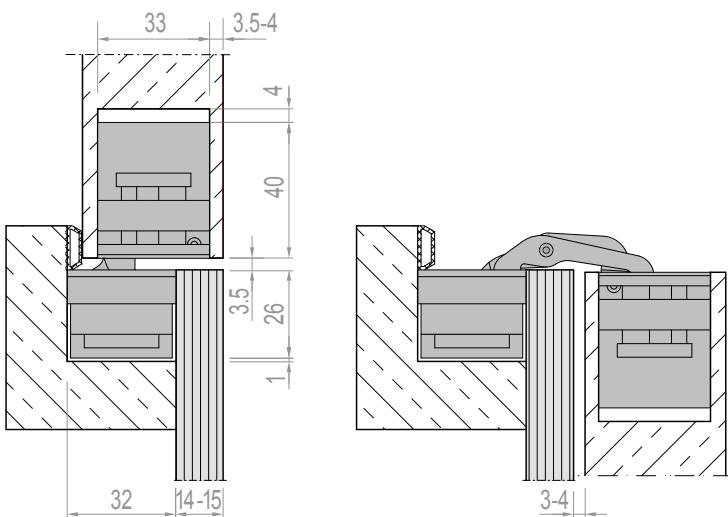
Section of Wood Frame-Door Installation
