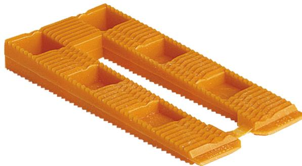
The Orange Wedge is often used for leveling of components on vertical surfaces, since it can be slid in between the wall and the item with a "leg" on each side of the screw, hence preventing it from falling down. The orange Wedge is also used for leveling of lighter components, temporary spacing etc. Due to the unique tooth pattern it can only be used with another Orange Wedge.
